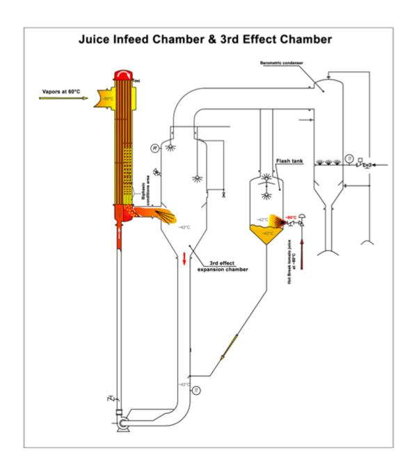
To avoid the "tomato juice carry over" into the condenser of the Evaporatos ZEUS having capacity above 1200ton/day, corresponding to 40000lt/hr of evaporated water, we add the Expansion Chamber receiving the HOT BREAK tomato juice at 80°C or more.
